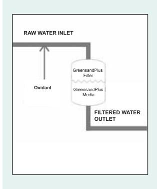
Catalytic Oxidation (CO) operation is recommended in applications where iron removal is the main objective in well waters with or without the presence of manganese. This method involves the feeding of a predetermined amount of chlorine (CI<sub>2</sub>) or other strong oxidant directly to the raw water before the GreensandPlus Filter.
