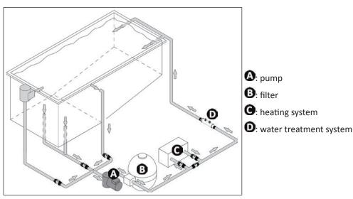
• Use as few elbow joints as possible. If there need to be more than 10 elbow joints on the hydraulic circuit, increase the pipe diameter.
