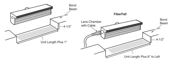
After notching the beam (setting blocks):
