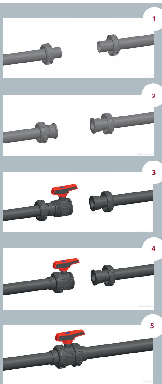
**SEAL-CARRIER****Industrial Series - Threaded seal-carrier**
